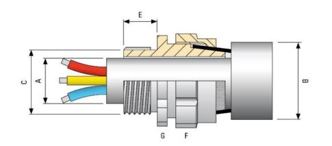
Designed to the B.S. 6121 standard, the IGBW is a robust metallic range of cable glands for industrial applications which provides armour clamping, grounding and earthing, with no IP seal.
